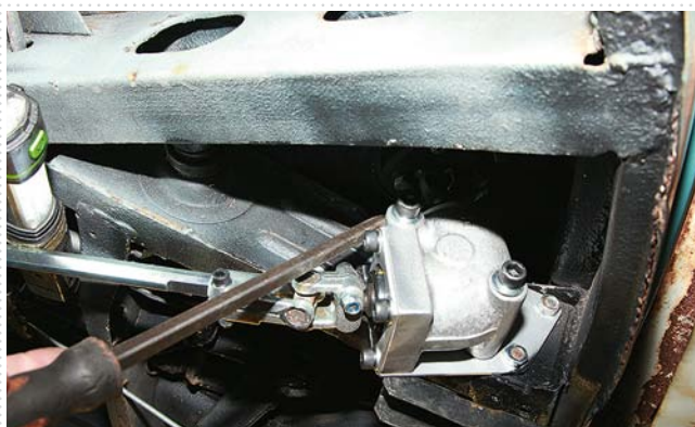
10 Lever down against the steering box to liberate the splined steering shaft from the coupling
