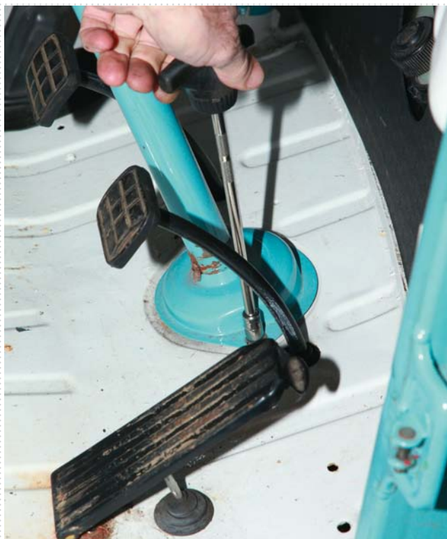
08 Next, undo the two bolts that retain the steering column outer casing to the cab floor...
