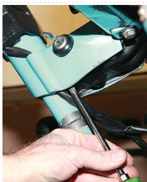
07 Undo the Phillips head screws that secure the cowling to the dash surround
