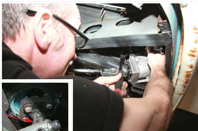
09 ...and undo the M8 pinch bolt that secures the steering column shaft to the steering box beneath the Bus
