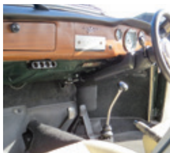
Once fitted, the steering column looks completely standard, an important point
